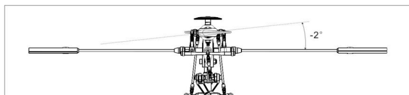
Stick position at low/Throttle 0%/Pitch 0° 摇杆低速/油门0%/Pitch 0°
